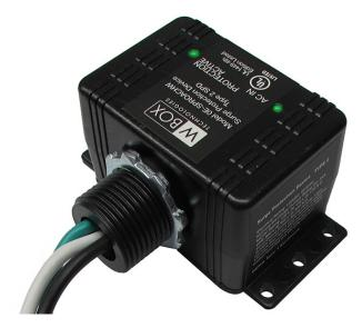
The high performance OE-SPROACHW is a Type 2 Surge Protection Device that protects sensitive electronic loads connected to service panels, intrusion alarm panels, fire panels and devices connected directly to it, via parallel installation on 120VAC branch circuits. LED indicators for AC input and active surge protection. NEMA Type 1 sealed ABS weather and impact resistant plastic enclosure. Lead wires 15". UL1449, 4th Edition listed.
