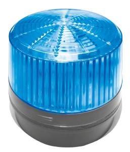
Model OE-STROBERPB is a high output, rainproof strobe suitable for both indoor and outdoor applications. Strobe life expectancy is 50,000 hours, up to 250 times that of comparable models. Mounts on bell box or other enclosure (including W Box model OE-STSTSIREN) or directly to wood or other surface. Two bolts, two nuts and two wood screws are provided. An adhesive mounting gasket is provided to enhance rainproofing. A rubber ring seals the lens with the base.
