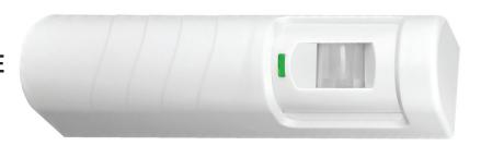
Model OE-RXD is a Request-to-Exit (REX) motion detector that detects motion within its adjustable coverage area via passive infrared (PIR) detector to provide door control via a door control device (such as magnetic lock or door strike) or access control system. A variety of programable options allows customization to suit the application. Durable ABS plastic housing. Optional trim plate (OE-TP) facilitates neat installation, especially with use of single gang box.
