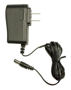
The OE-PPS12V1AC is a fully regulated 12VDC, 1 amp plug-in switching adapter that provides reliable DC power for a wide variety of indoor security and surveillance products and applications. It can be used with input voltage ranging from 100 to 240VAC and includes a power indicator LED. Self-limiting protection against short circuit and overload conditions is included, with auto recovery. Complies with DOE Level VI Efficiency and FCC requirements.
