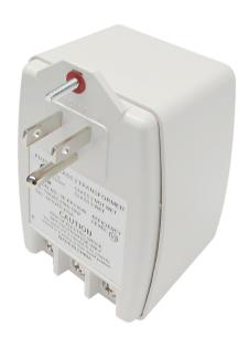
The OE-PPS2440 is a plug-in 24VAC, 40VA plug-in transformer that provides reliable AC power for a wide variety of indoor security and surveillance products and applications. It is auto-resetting PTC fuse protected and includes a power indicator LED. Grounding is provided via a third screw terminal and ground plug. Complies with DOE Level VI Efficiency requirements for alarm industry plug-in power supplies.
