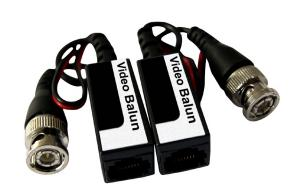
Single-channel passive video balun enables full motion video transmission and power transmission over UTP up to 2,000', or 3,000' if used with an active receiver. Compatible with analog or HD. Easy installation with RJ45 jack, pigtail BNC connector and power wires. One pair per package.
