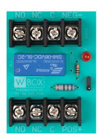
Applications include intrusion, access control, video surveillance and other systems requiring control or activation of electronic devices. Operations include dry contacts, latching dry contacts, polarity reversal and line seizure. Includes double-sided foam mounting tape.
