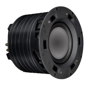
Rich, deep bass from a compact, 'Integrated Back Box' utilizing Sonic Vortex® technology. This patented technology is a 'twist' on Ported Transmission Line design, that doubles as a built-in back box to keep speaker sound from bleeding to other rooms while adding 6 to 9dB boost in mid-lower bass for solid bass response. Recommended crossover at 80Hz and below.
