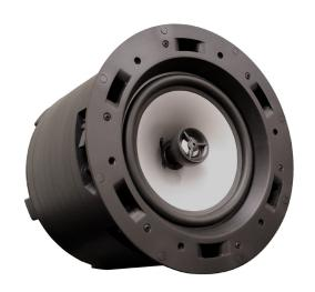
Rich, deep bass from a compact, 'Integrated Back Box' utilizing Sonic Vortex® technology. This patented technology is a 'twist' on Ported Transmission Line design, that doubles as a built-in back box to keep speaker sound from bleeding to other rooms while adding 6 to 9dB boost in mid-lower bass for solid bass response.
