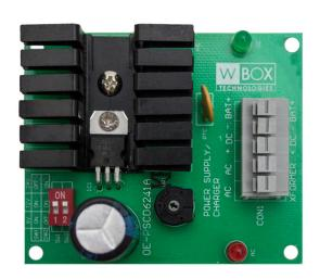
Converts low voltage 16.5VAC or 24VAC input (typically a plug-in transformer, not included) into 6VDC, 12VDC or 24VDC output. Battery charger output with automatic switchover to DC upon AC failure. Applications include intrusion, access control, video surveillance and other low voltage systems requiring extra power. Includes double-sided foam mounting tape and battery lead wires.
